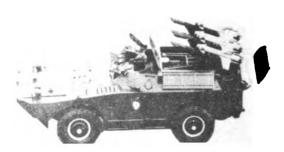
Figure 6-37 AT-2 SWATTER. SWATTER missiles appear in a quadruple mount on a modified BRDM. Shown here is the launcher raising sequence.
